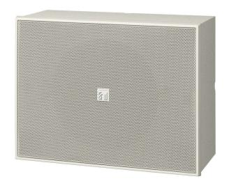
The BS-678E, of which cabinet is made of wood, can be installed in a vertical or horizontal orientation. Either concealed in-wall wiring or exposed wiring can be used for speaker cable connection. The speaker structure that permits direct wall-mounting with screws prevents the speaker from falling easily even if an outward force is applied to. Two built-in 6 inch double cone speaker units deliver high quality sound.
